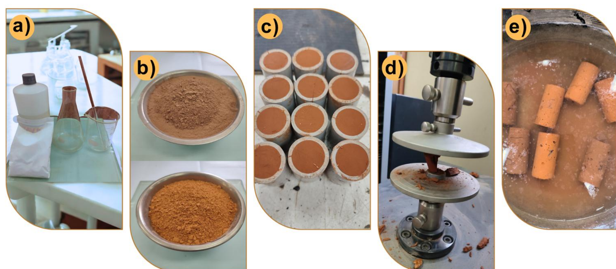
Figure 2: (a) Alkaline activators; (b) brick and ceramic waste powders; (c) preparation of geopolymeric specimens; (d) compressive strength test; and (e) density, absorption, and voids tests.
