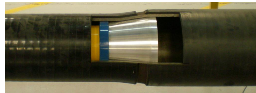
Figure-2 Cutaway section showing expansion cone (mandrel) and aligner
