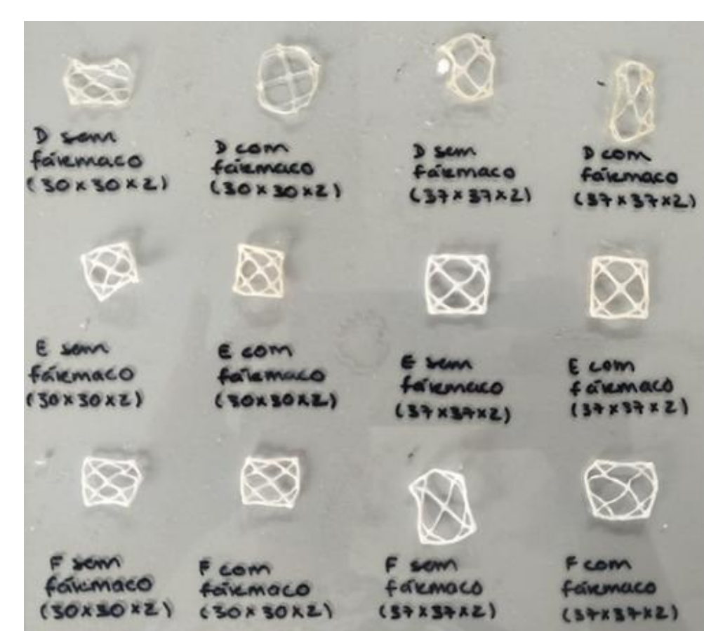
Figure 4 – Visual aspect of some structures after chemical crosslinking.
