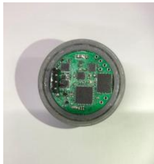
Figure 2. Demonstration of the instrumented particle showing the MEMS sensor encapsulated with the 3D printed waterproofed casing (with external diameter of 3cm). [2]
