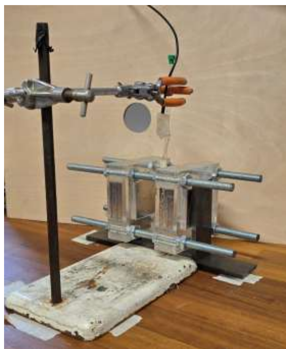
Figure 4. Photograph of variable field sensor showing variable position magnet housings and suspended RF coil and sample.
