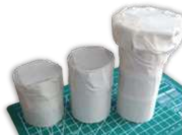
Figure 3. Sample target objects used for dataset generation, from left to right: heights of 5 cm, 7 cm, and 9 cm; cross-sectional areas of 20 cm 2 , 20 cm 2 , and 40 cm 2 , respectively.
