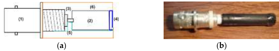
Figure 6. Design of the piezoelectric acoustic detector, (a) model; (b) real PAD.
