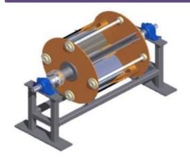
This study addresses this challenge by evaluating the scale-up of a TiO<sub>2</sub>-based rotary concentrator photoreactor (RCPR) specifically engineered for the photocatalytic degradation of cyanide in contaminated water.
