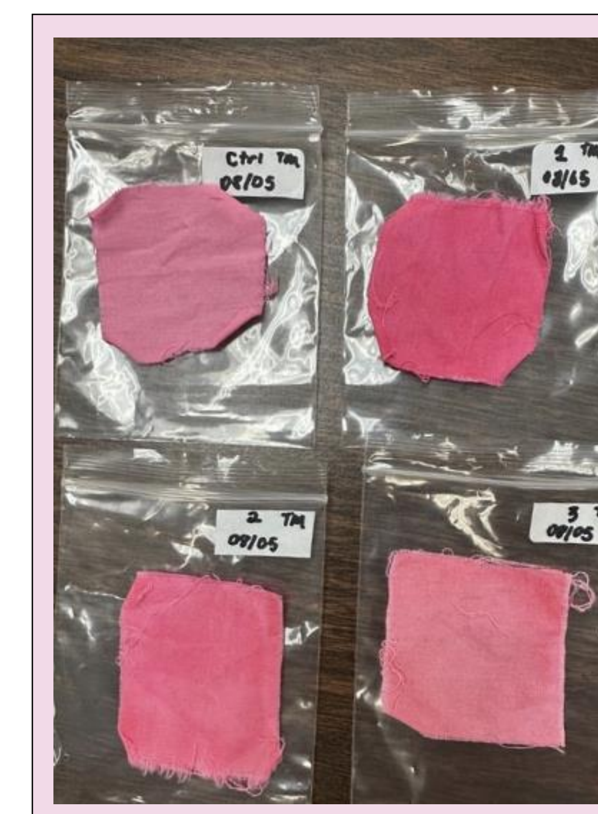
Figure 1. Cotton fabric dyed with the photocatalyst Eosin Y, showing the characteristic pink coloration after immobilization.
