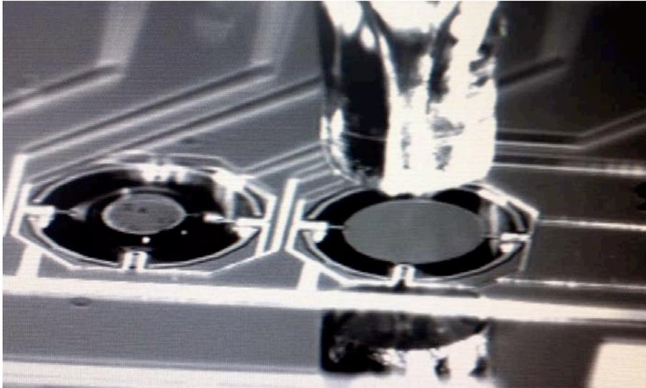
Total dispensed amount per MSS: 6 nL polymer solution in water (1mg/mL)
