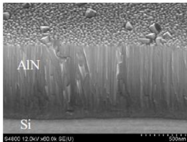
Figure 1. Left: scanning electron microscope (SEM) picture of the texture gradient of an AlN film; right: schematic cross section of a thin nanocrystalline aluminum nitride film.
