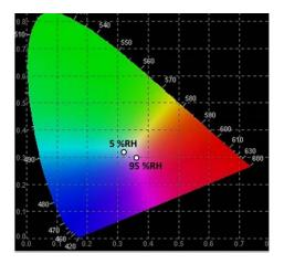
**Figure 5.** CIE color coordinates for polymer films with thickness of 290 nm deposited on 5-layers Bragg stack comprising SiO₂ and Nb₂O₅ films at denoted values of relative humidity.
