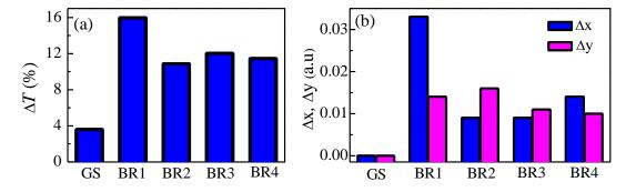
**Figure 4**. Humidity induced changes in transmittance (a) and CIE color coordinates x and y (b) for single polymer film with thickness of 290 nm deposited on bare glass substrate (GS) and on Bragg reflectors (BR) (BR1-5 layers, BR2-7 layers - Nb<sub>2</sub>O<sub>5</sub> and SiO<sub>2</sub>; BR3-5 layers, BR4-7 layers - dense and mesoporous Nb<sub>2</sub>O<sub>5</sub>).
