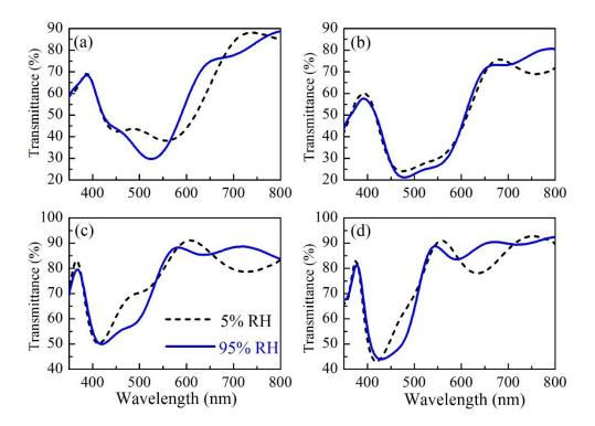
**Figure 3.** Transmittance spectra at low (5%) and high (95%) relative humidity of branched polymer film with thickness of 290 nm deposited on top of Bragg reflectors consisting of 5 (a, c) and 7 (b, d) alternating layers of Nb<sub>2</sub>O<sub>5</sub> and SiO<sub>2</sub> (a, b) and dense and mesoporous Nb<sub>2</sub>O<sub>5</sub> (c, d)
