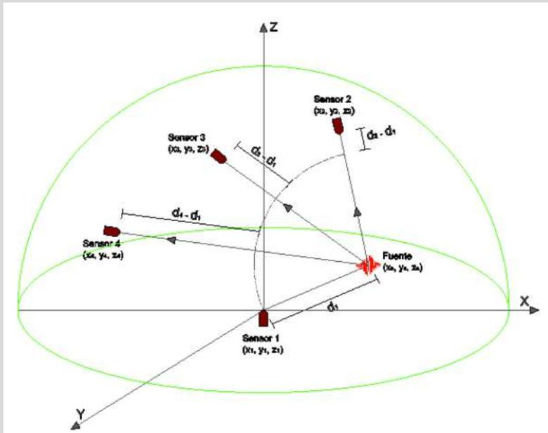
A general model for three dimensional (3-D) estimation of a source using  $M$  receivers is developed. To obtain the location of the source, we start by knowing the spatial position  $(x_i, y_i, z_i)$  of a certain number of sensors  $N$  ( $i = 1, 2, \dots, N$ ). Let  $(x_s, y_s, z_s)$ , the position of the source to be located, **the distance between the source and the  $i$ -th sensor** will be:
