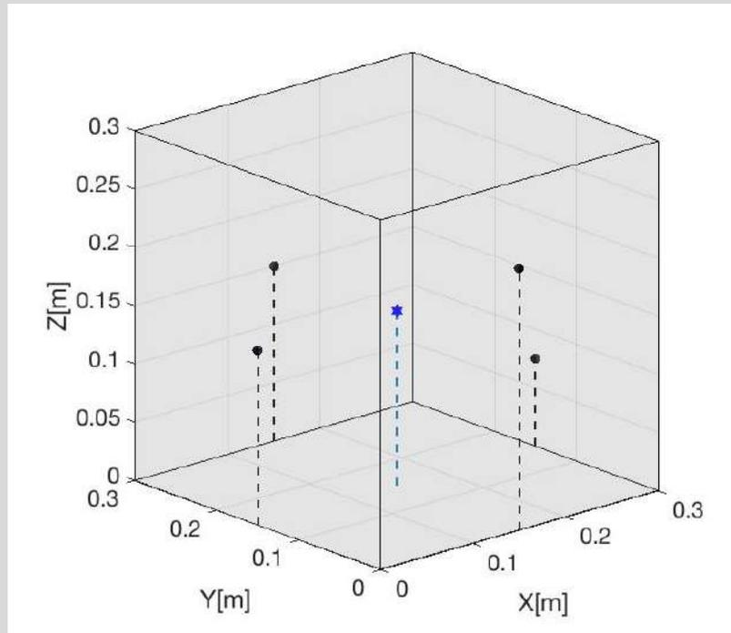
To evaluate the algorithm, the volume of the cube has been modified between  $27.0 \cdot 10^{-3}$  to  $512.0 \cdot 10^{-3} m^3$ . The positions of the sensors are shown in the table where  $H$  represents the size of the edges, that is, values of edges were 200, 300, 400, 500 and 600 mm.
