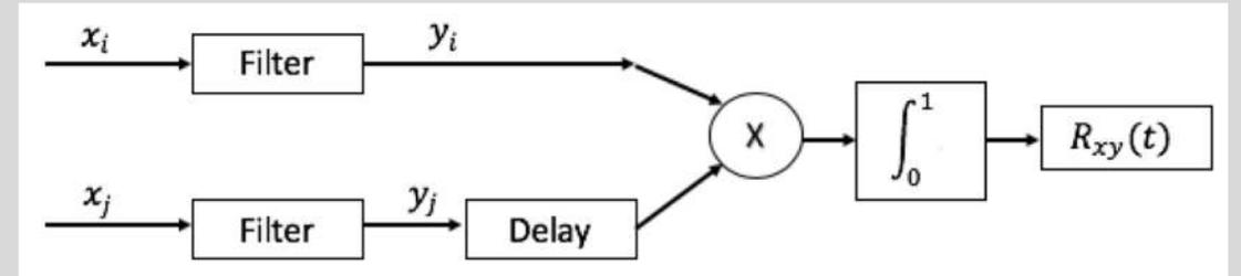
Where  $R_{x_i x_j}$  is the **cross-correlation between the signal  $x_i$  and  $x_j$  filtered by the filters  $H_i$  and  $H_j$** , is expressed as a function of the power spectral density  $G_{x_i x_j}$
