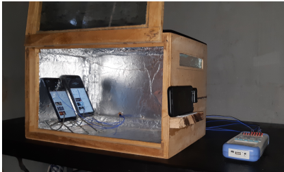
Test chamber with the mobile phone setup.
