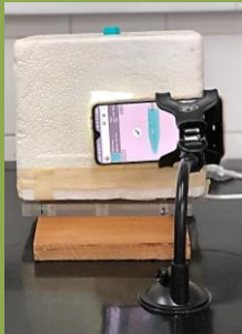
Styrofoam box with LED lamp and smartphone holder
