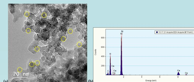
Characterization of Si/SiO<sub>2</sub> QDs by TEM (a) and EDXS (b) investigations. Note the spherical shape of QDs marked by yellow dot circles (a).
