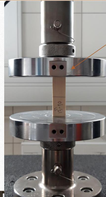
Compressive strength along the fibres ( $Rc_{12}$ ) was determined using an Instron 3382 machine.
