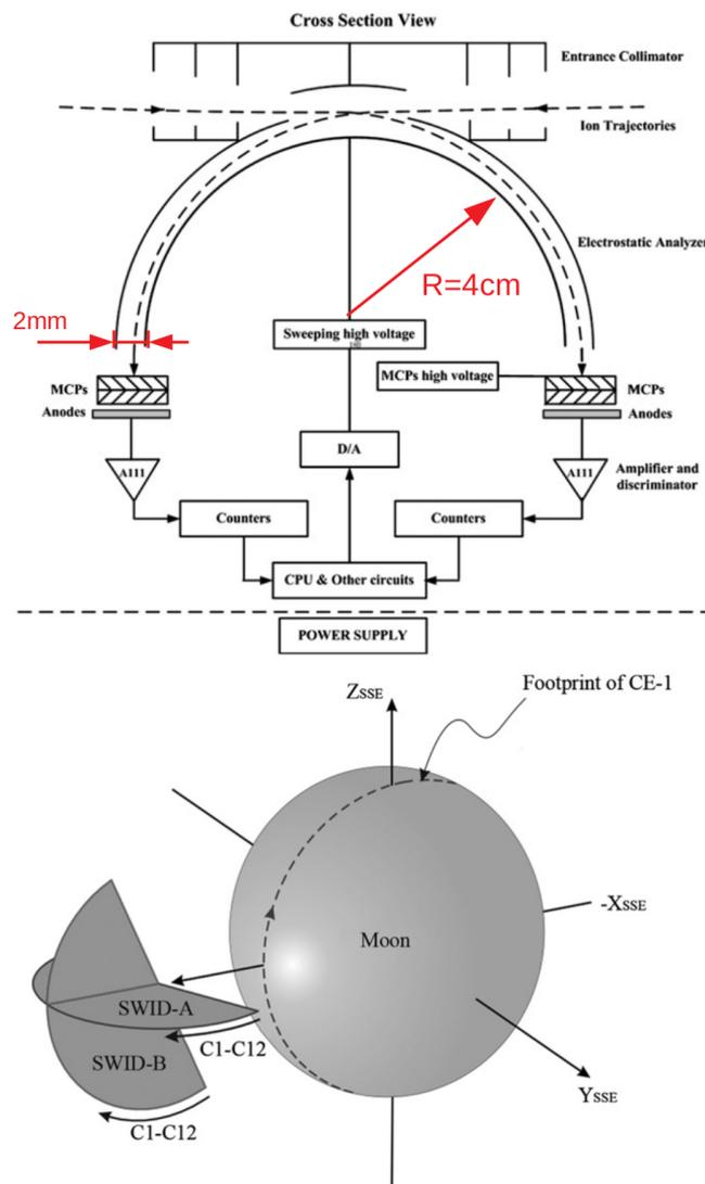
**Figure 1.** Basic principle diagram of SWID. The orbit of the Chang'E-1 spacecraft allows to scan a large fraction of the sky in the field of view of the SWIDs.
