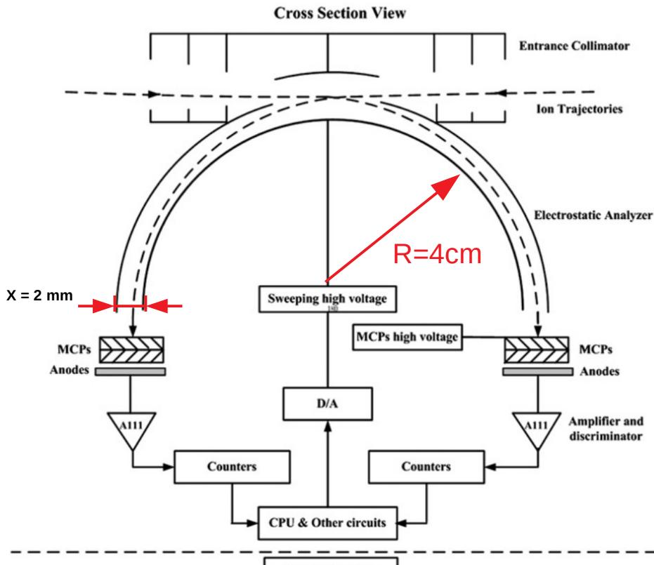
MCPs anode segmented in 12 channels
