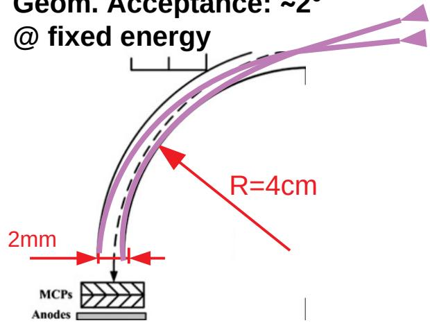
detector response calibrated @ 5eV-800eV ion beam
