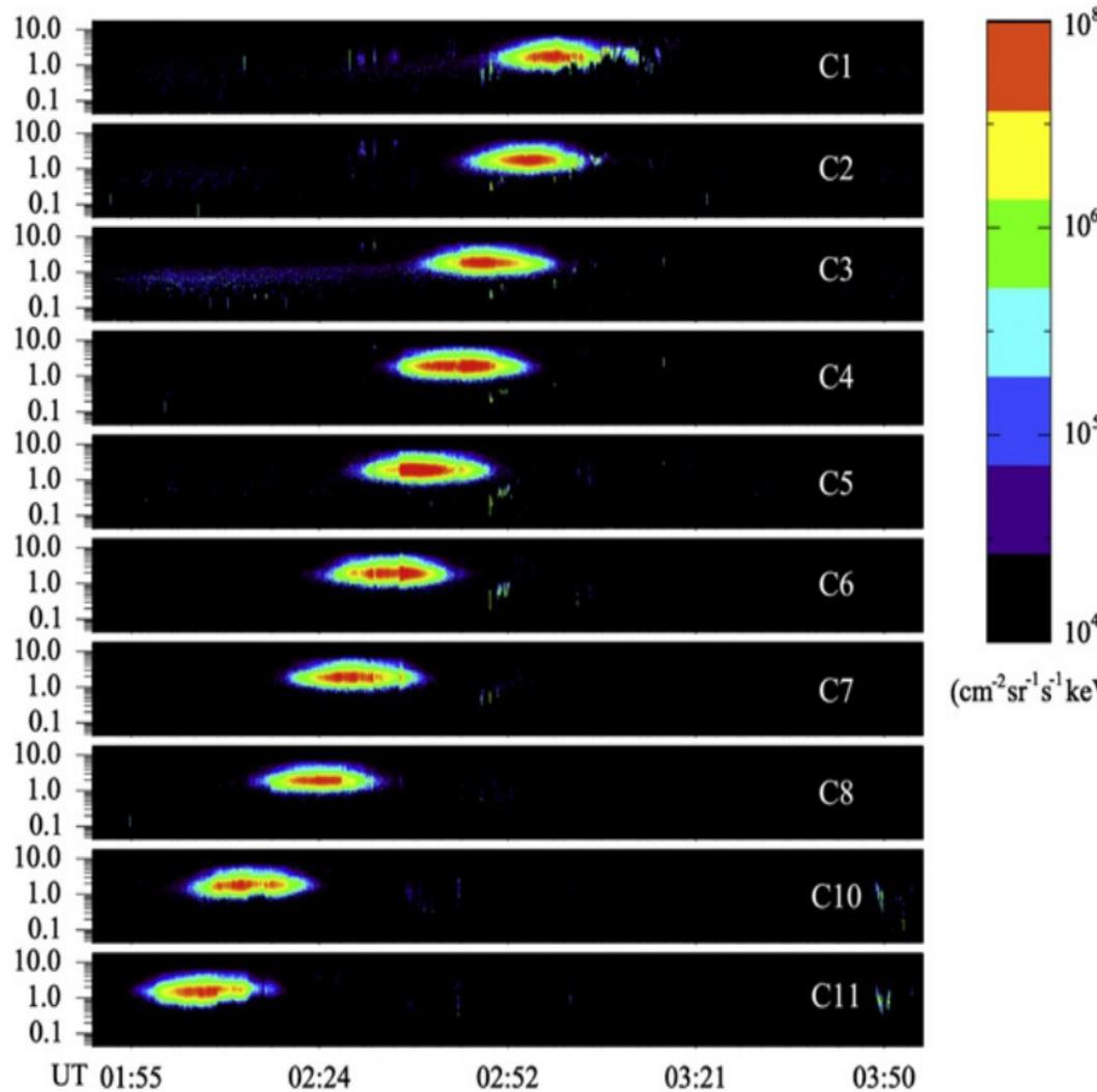
When the SUN (i.e. the solar wind) enter in the acceptance of a given channel, a large flux is measured.
