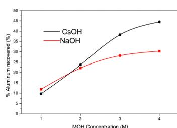
Percentage of recovered aluminum for different alkaline hydroxide concentrations
