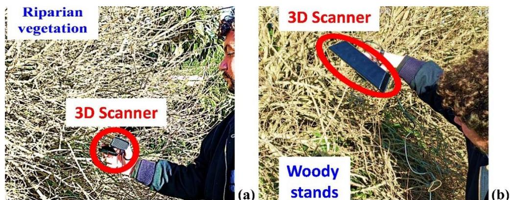
**Figure 2.** Examples of 3D scans associated with rigid riparian vegetation covering vegetated drainage channels: (a) Frontal and (b) Above scans of vegetation canopy and stems. The red ellipse indicates the 3D scan sensors.
