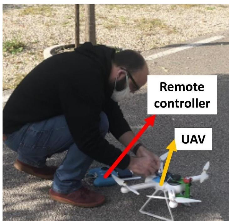
**Figure 3.** View of UAV used in this work. The yellow and the red arrows indicate the UAV device equipped with a multispectral camera and the remote controller, respectively.
