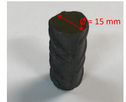
Carbon steel sample
