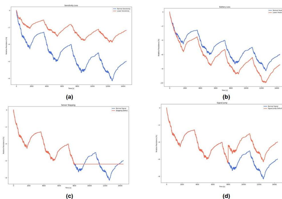
**Figure 4.** Different Signal Outputs for the different sensor fault types implemented in the stochastic model. (a) Sensitivity Loss (b) Battery Loss (c) Sensor Stopping (d) Signal Jumps.
