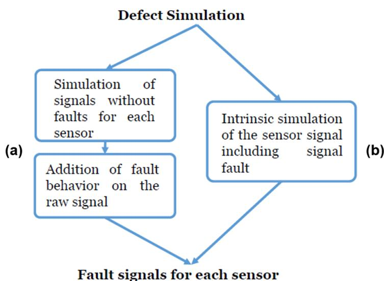
**Figure 3.** Different Approaches for the Sensor Fault Model. (a) shows a post-simulation approach, where the faults are added after the sensor signal was simulated by the Sensor Response Model. (b) shows the intrinsic simulation approach, where the fault behavior is integrated in the Sensor Response Model.
