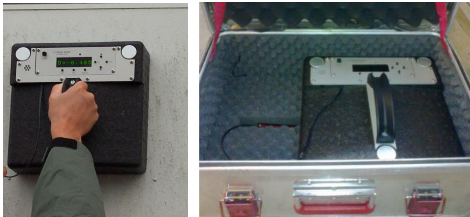
Figure 1. U-value measurement on outer wall. The figure also shows an insulated acclimation suitcase, in which the meter is placed in between the individual measurements.
