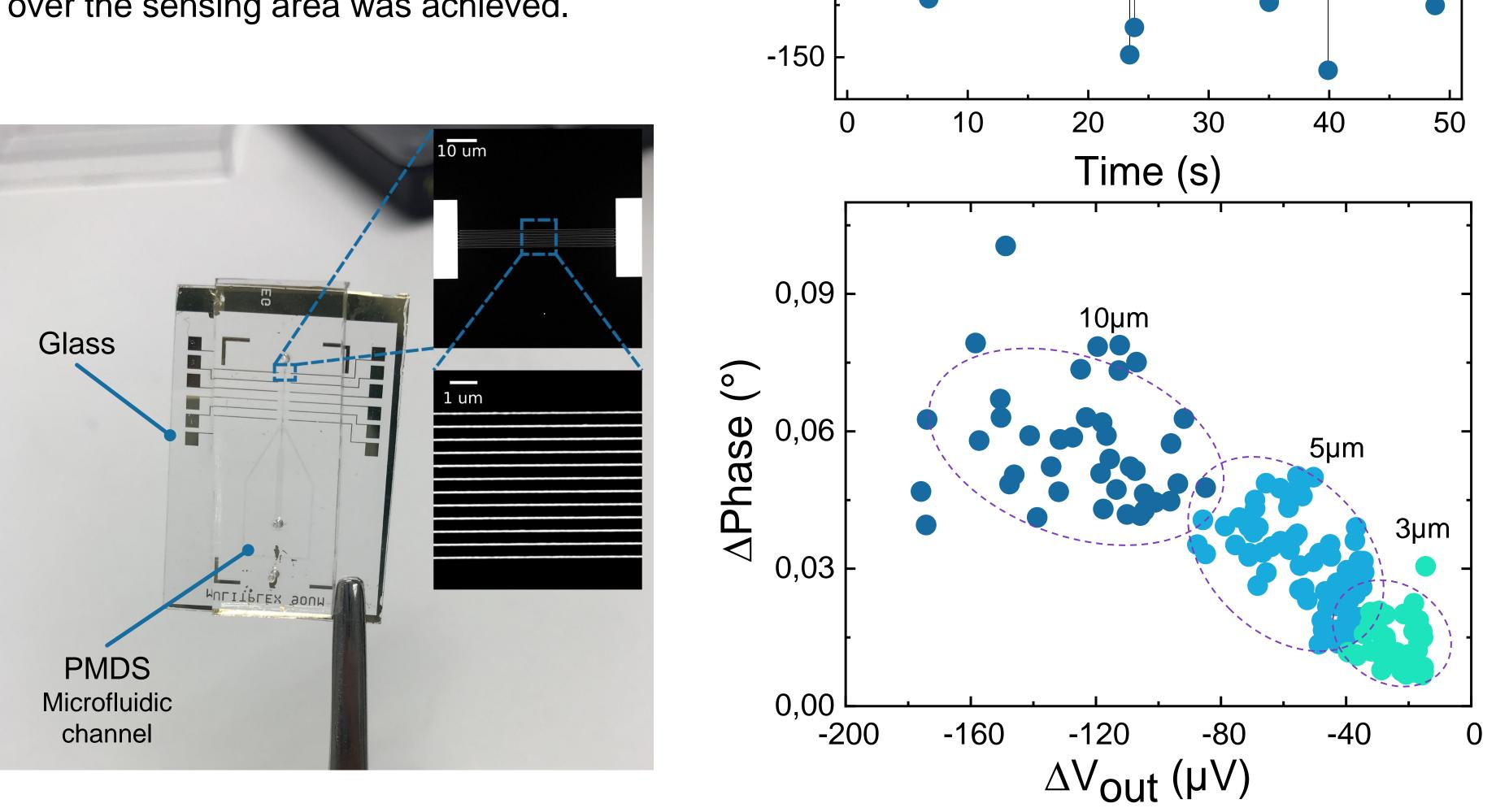
tested with the impedimetric was μm) platform. The signal change induced by a particle passing over the sensing area is sizedependent. Particles of 3  $\mu$ m, 5  $\mu$ m, and 10  $\mu$ m show a mean  $\Delta V_{out}$  of -19  $\mu$ V, -52  $\mu$ V and -108  $\mu$ V, and a mean  $\Delta$ Phase of 0.015°, 0.03° and 0.06°, respectively.
