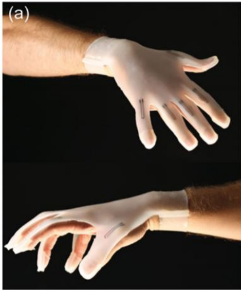
Deformation sensor based on resistive ink from carbon in elastomer [1]
