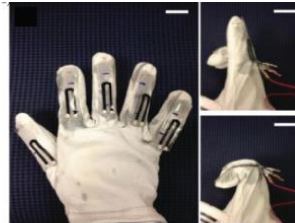
Photographs of gloves with five sensors made of graphene oxide and nanocellulose, changes in the resistance of five independent strain sensors [3]
