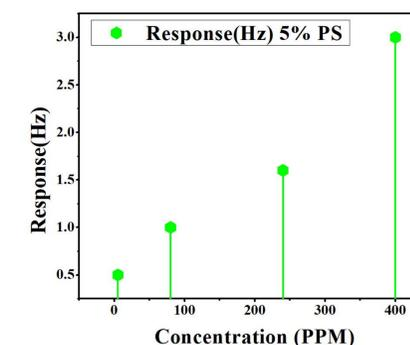
Figure 5: Sensor response for varying concentrations of ACT
