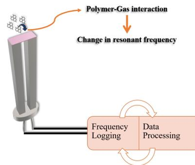
Figure 2: Sensing Methodology
