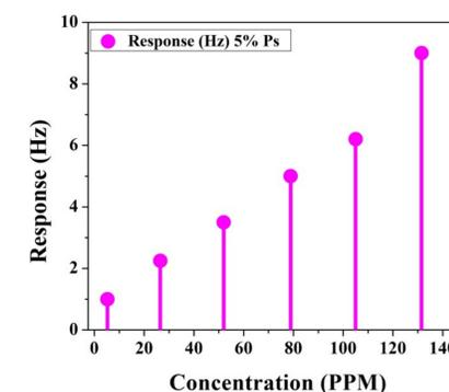
Figure 4: Sensor response for varying concentrations of PBZ
