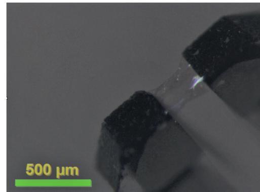
Figure 1: Polymer (Polystyrene) film placed on the tines of the QTF
