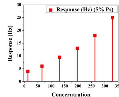
Figure 3: Sensor response for varying concentrations of STY
