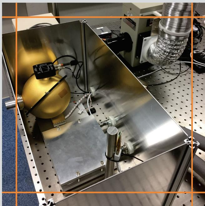
Afterward, the integration sphere output is directly attached to the cryostat, which is containing the detector to be characterized.
