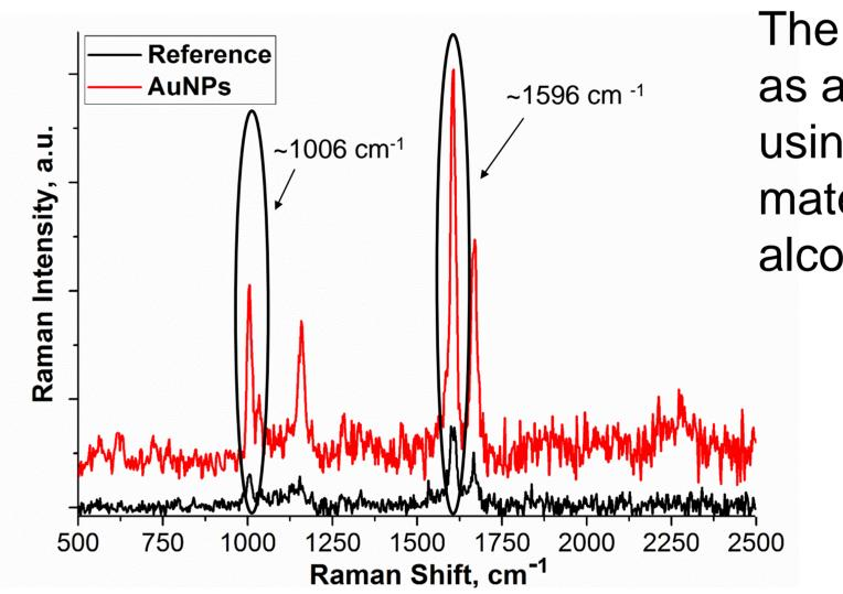
The SERS enhancement was calculated as an analytical enhancement factor using two peaks of the investigated material, benzophenone-izopropyl alcohol solution :
