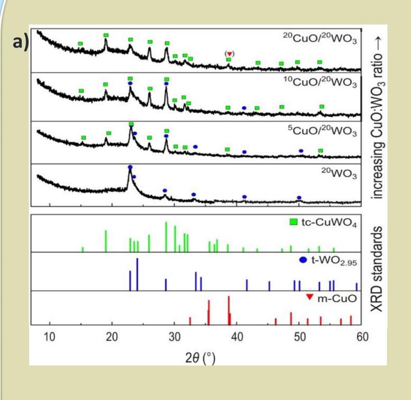
As deposited WO<sub>3</sub> thin films, CuWO<sub>4</sub> loaded WO<sub>3</sub> (a), Pd Loaded HiPIMS deposited WO<sub>3</sub> measured film up to 350 °C, (colored curves in (b)) and Change in Stoichiometry with Voltage Pulse length (c).
