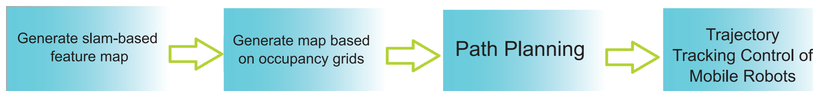
Figure 3: Algorithm for path planning of mobile robots.
