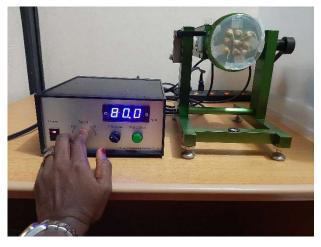
**Figure 1.** 2-D Clinostat at the Microgravity Simulations Laboratory, National Space Research and Development Agency (NASRDA), Abuja, Nigeria.
