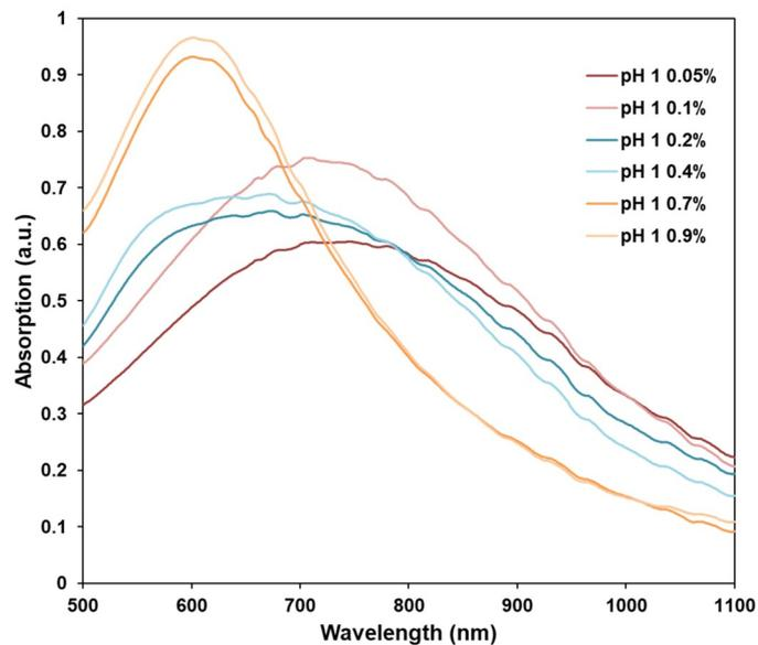
Figure 2. UV-Vis absorption of AuNS.
