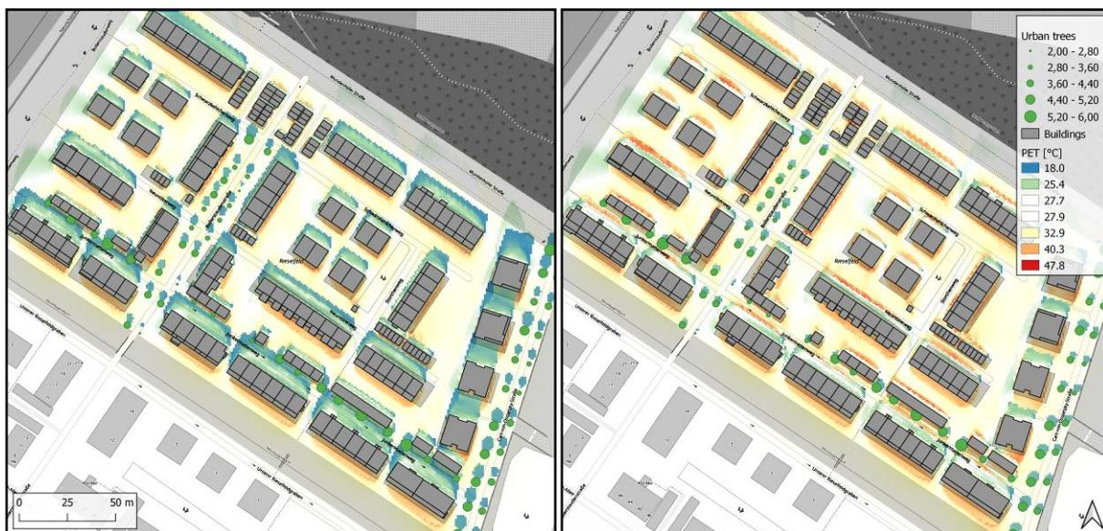
**Figure 4.** Thermal comfort, based on PET in 1.1 m above ground level for a residential neighborhood in Freiburg, Germany at 13:00 LST, 1st of April (left) and 1st of July (right)
