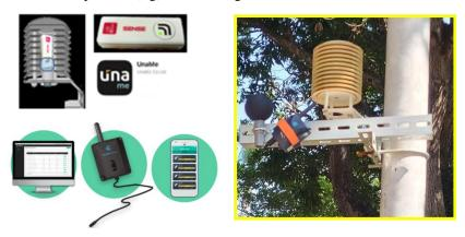
Figure 3. UnaSense (left up) and Temphawk (left down) sensors and the installation.
