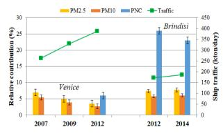
**Figure 4.** Relative contribution of particles' concentration in previous campaigns in Venice and Brindisi, with indication of ship traffic volume [21,23]. Results for PM<sub>10</sub> from indirect calculation obtained considering a ratio PM<sub>2.5</sub>/PM<sub>10</sub> equal to 0.78.
