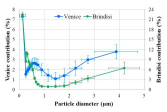
**Figure 3.** Relative contribution of shipping to number particle concentration as function of size for the two sites, during the last campaigns in 2014 (Brindisi) and 2018 (Venice) [15]. Vertical bars represent the errors and horizontal bars the size of the channel used in the evaluations.
