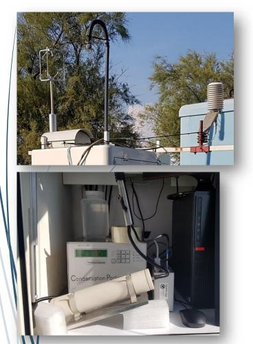
ECAS 2021 \*CPC Condensation Particle Counter OPC Optical Particle Counter
