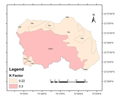
erodibility factor map prepared which shown in Figure 6, which shows the maximum value 0.3 for loamy soil 0.22 for clay soil. The range of K value varies between 0 to 1.
