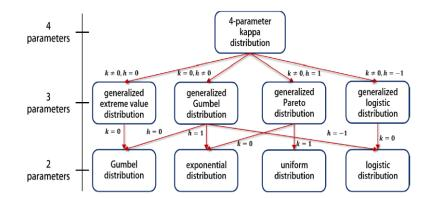
**Figure 1.** Relationship of the four parameter kappa distribution (K4D) to other distributions, which indicates a wide coverage of K4D.
