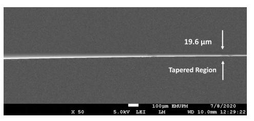
(SEM) micrograph of the transition region of the prepared tapered multimode optical fiber (MMF)
