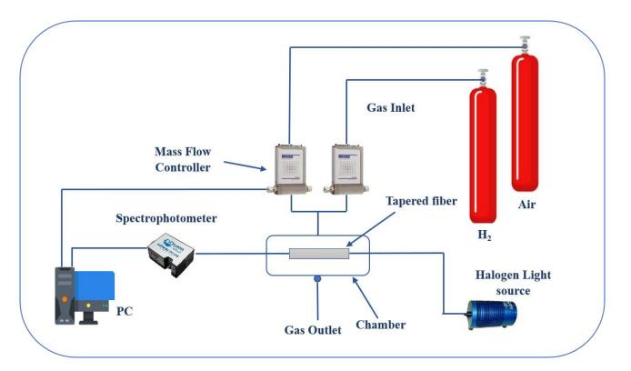
The experimental setup of the  $H_2$  sensor.
