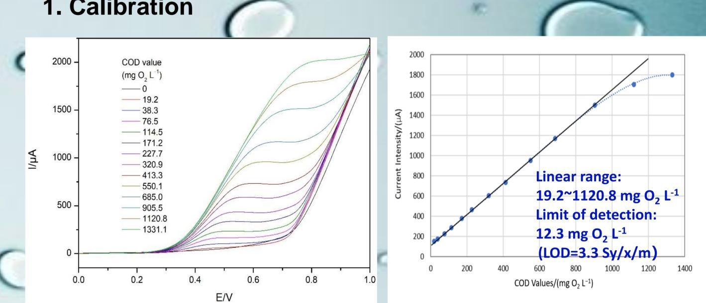
Figure 4. (A) Oxidation curves of cyclic voltammetric responses of electrode **E1** with the increase of addition of glucose in 0.05 M NaOH solution. (B) Calibration plot of intensity of current at E=0.7050 of electrode **E1** as a function of COD values (glucose as standard substance). Potential scan window, -1.0 to +0.7 V vs. Ag/AgCl (3.0 M KCl). Scan rate, 50 mV/s.
