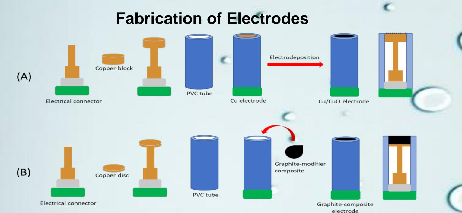
Figure 1. Diagram of the fabrication procedures of (A) the deposited Cu/CuO electrode and (B) the graphite-epoxy electrodes (E2, E3 and E4) modified with metal nanoparticles (Cu, CuO and Ni Cu alloy, respectively)
