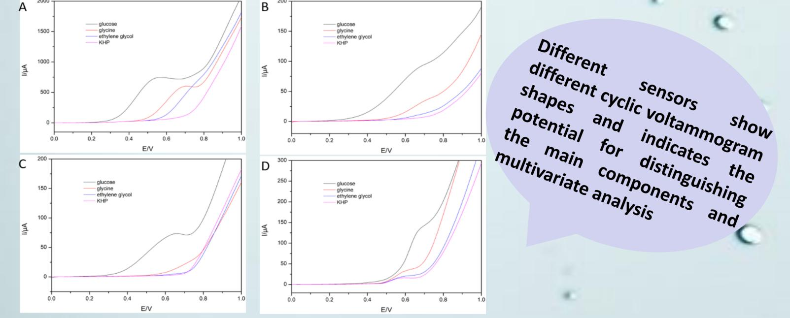
Figure 2. Oxidation curves of cyclic voltammetric responses of electrodes E1 (A), E2 (B), E3 (C), and E4 (D) to four standard chemical oxygen demand (COD) substances: 2.15 mM glucose; 2.15 mM glycine; 2.15 mM ethylene glycol; 2.15 mM KHP.
