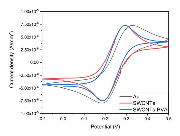
Modified electrodes presented similar current density and a smaller potential gap than Au bare electrodes
