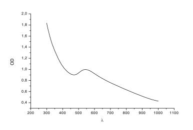
Absorption spectra of Au nanoparticles embedded in glycan matrix
