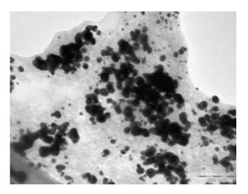
TEM image of Au nanoparticles embedded in glycan matrix
