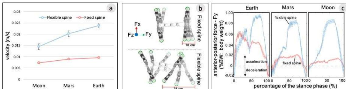
**Figure 2.** (a) Robot locomotion speed compared between movements with flexible and fixed spine modes on Earth, Mars, and the Moon. (b) Stride length of the robot both with and without a flexible spine. (c) Comparison of GRFs ( $F_y$ ) for fixed and flexible spine movements under three gravitational scenarios.
