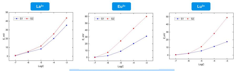
Potentiometric response curve for REMs at pH=2
