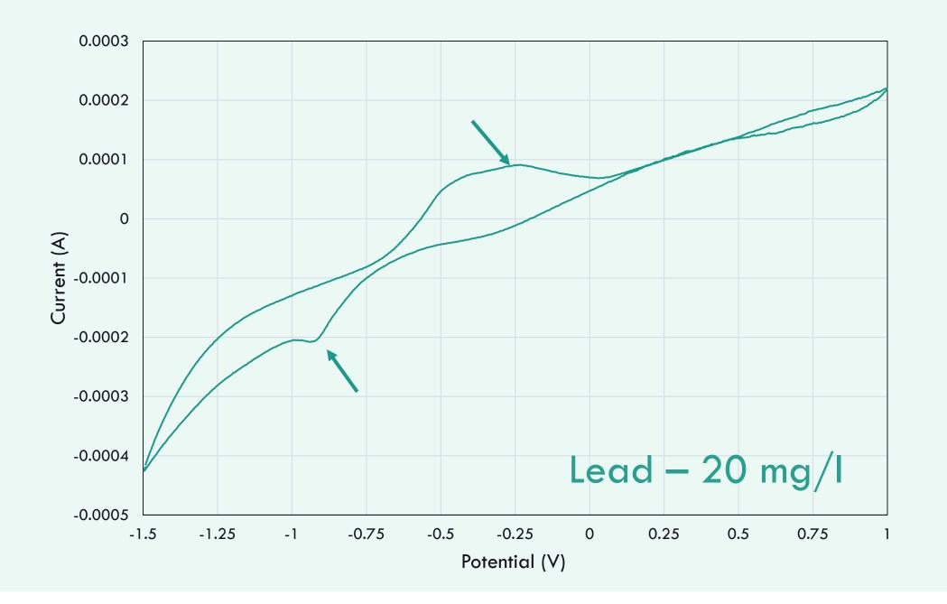
The results of cyclo-voltammetry measuraments showed typical peaks related to the two metals present individually in the solution.
