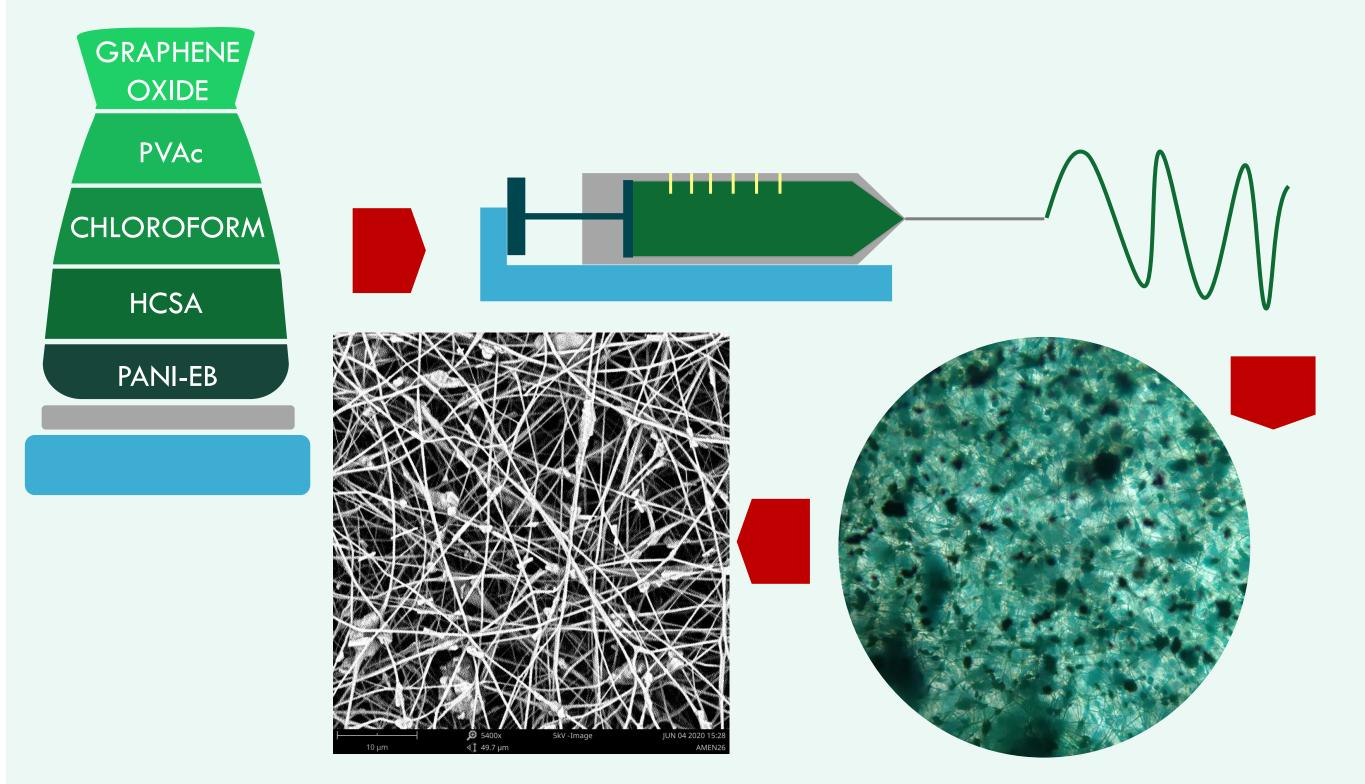
Nanofibers were collected using the electrospinning technique. This technique allows to spin a polymer solution through the use of a high potential electric field. Electrospinning solution was obtained dissolving camphor-10-sulfonic acid (HCSA) and polyaniline emeraldine base (PANI-EB) in chloroform. Poly (vinyl acetate) and graphene oxide were then added in the solution.
