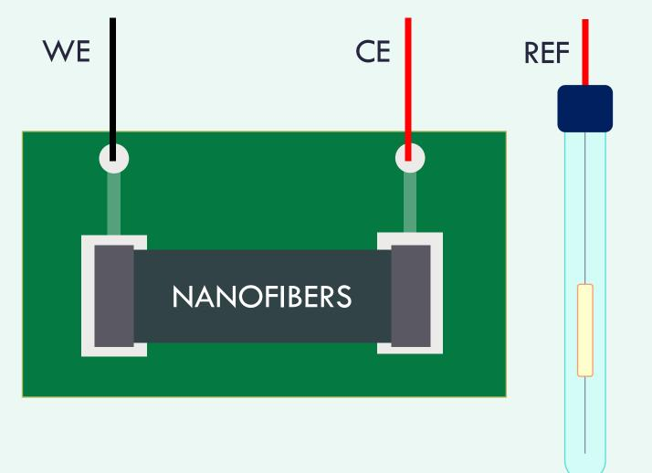
Printed circuit board (PCB) was used as a base to create a sensor, welding nanofibers to the two electrodes. Cyclo-voltammetry measurements were carried out using a AMEL 7050 potenziostatic/galvanostatic, with a potential in the range -1.5 V to 1,0 V and a scan rate of 50mV/s. Three-electrode setup was used to realize the measure, dipping them in a buffer solution with lead or cadmium iones.
