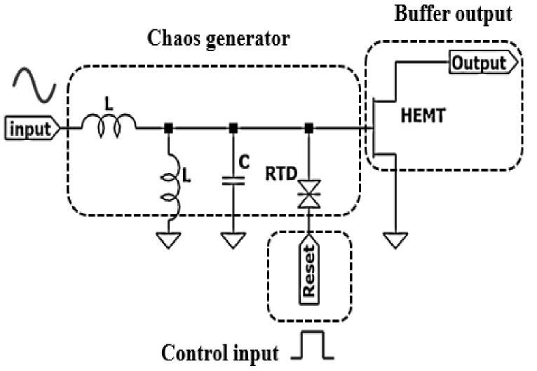
At pulse OFF state, circuit nonlinearities become weaker, which outputs sinusoidal signal
