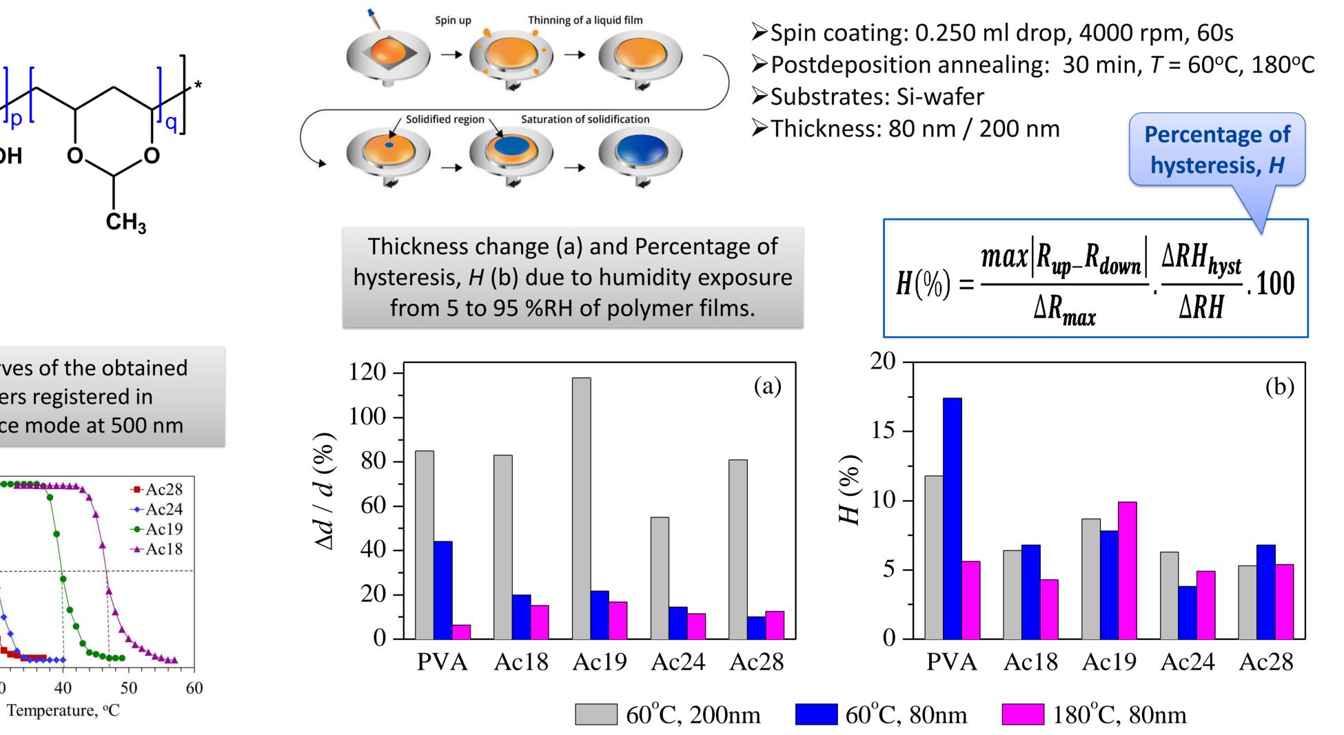
> Obtained poly(vinylalcohol-co-vinylacetal)s are smart materials exhibiting reversible phase transition in aqueous solution with increasing temperature. The higher the acetal content, the higher the hydrophobicity and the lower the phase transition temperature.
