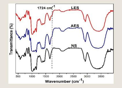
A new peak in the modified starches was observed at  $1724 \text{ cm}^{-1}$  representing C=O stretching group and it confirms the esterification modification by two organic acids.
