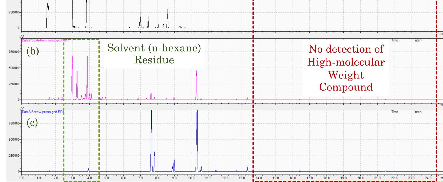
**Figure 1.** The GC chromatograms of (a) *n*-hexane, (b) Oil obtained from Soxhlet extraction of milled raw seed  $(Oil_{SE})$ , and (c) the extracted oil obtained from a screw-press machine  $(Oil_{SM})$
